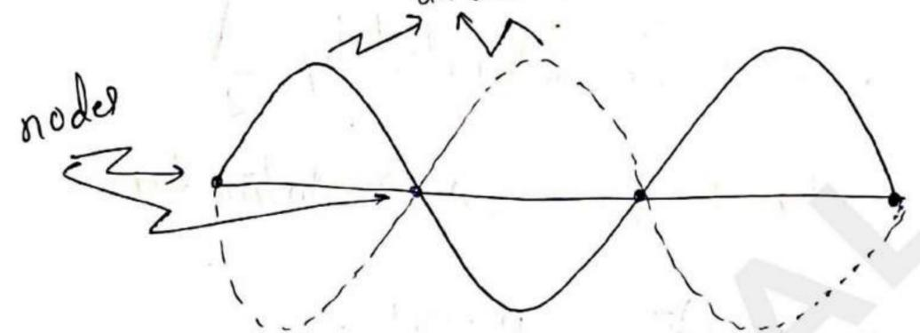
nodes - particles are stationary antinodes - particle executing motion with maximum amplitude.
