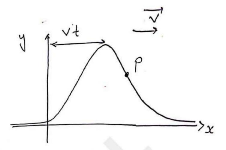
y(x,t) = f(x-vt)when wave move in +x direction y(x,t) = f(x+vt)when move move in -x -direction
