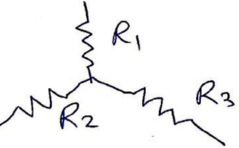
Kirchhoff's laws: -> Sum of potential difference across each component in a circular loop Zero I2R3+ I1R2=0 going from low potential to high potential side on buttery -> re (When going positive to negative side) IR (when move opposite to current) - IR ( when going along the lyment)
