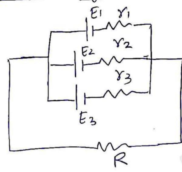
$$E_{eq} = \sum \left(\frac{E}{\gamma}\right) = \frac{E_1}{\gamma_1} + \frac{E_2}{\gamma_2} + \dots$$
