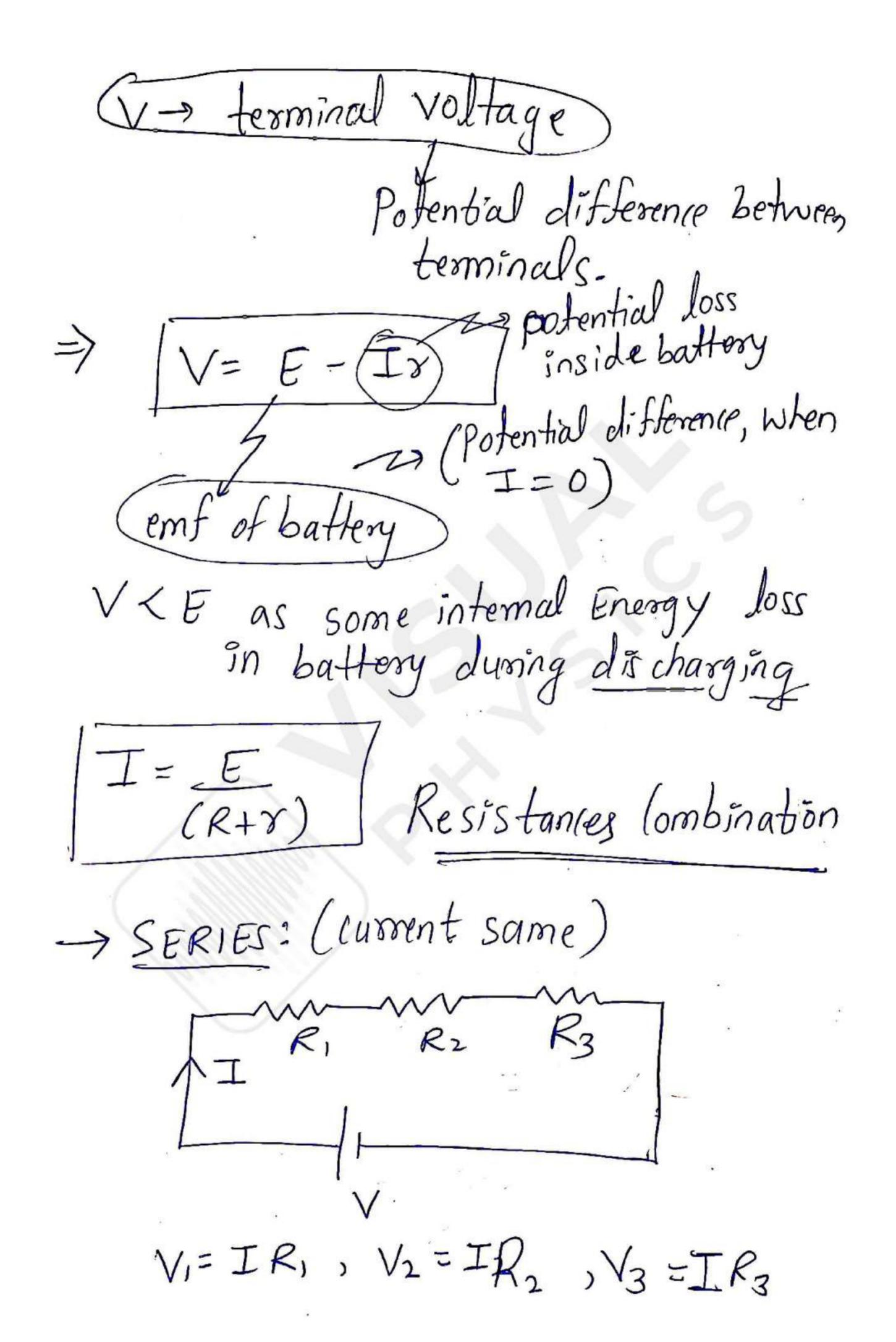
$$\Rightarrow IRnet = I(R_1+R_2+R_3)$$
