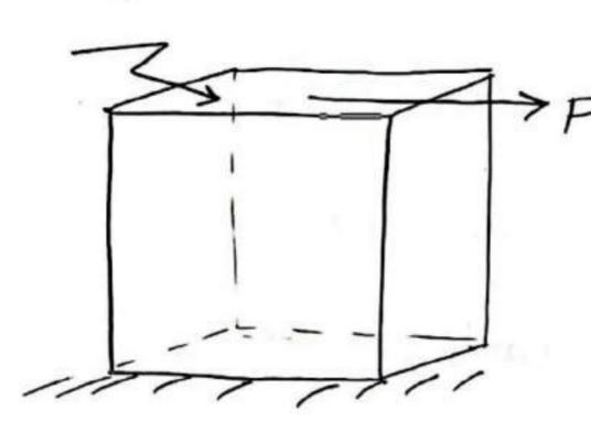
\* Fone acting tangentially to the surface \* deformation along the force, no change in volume.
