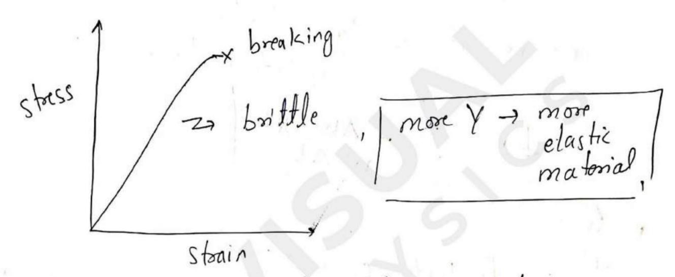
Implies more tougher material. Means more energy per unit volume is required to break the material.
